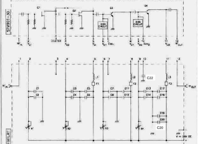
capable of 500mA full scale. 5) Note current draw before any adjustments are made. (Io) 6) Adjust R1 for lo + 100mA 7) Adjust R2 for lo + 280mA 8) Adjust R3 for lo + 330mA 9) Adjust R4 for Io + 480mA
